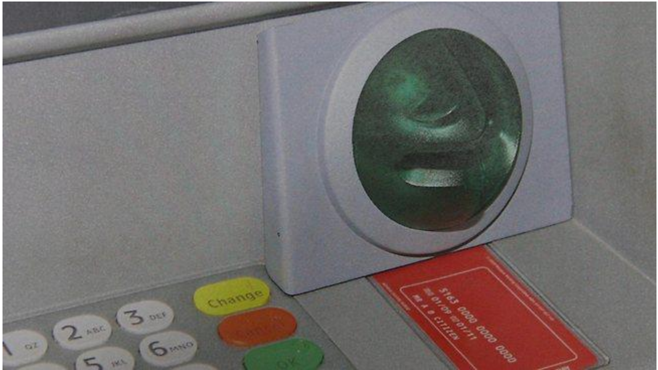
ATM card skimming device attached to ATM machine.
